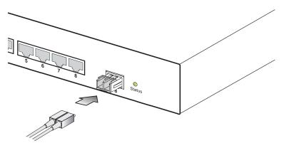
Figure 4-3 Making Connections to SFP Transceivers
